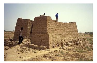
Figure 2: A brick clamp kiln is shown near Kassala. Photo: Theo Schilderman / Practical Action.
