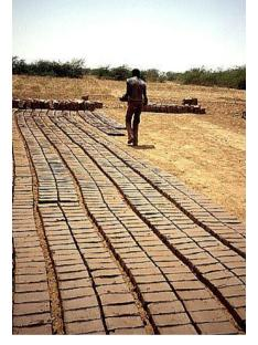
Figure 1: Moulded bricks pre-drying in the sun before being fired near Kassala. Photo: Theo Schilderman / Practical Action.
